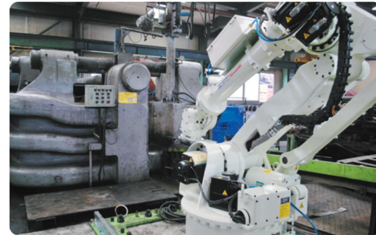
7.5 inch Upsetter Line
