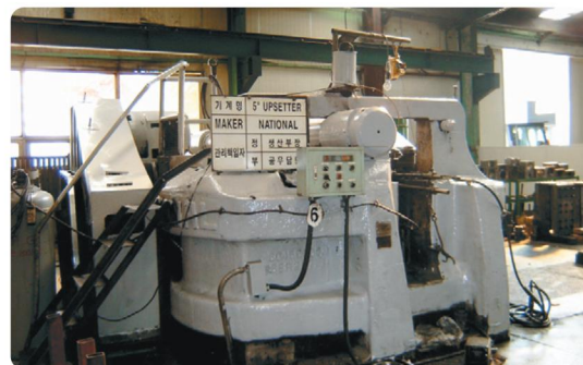
5 inch Upsetter Line
